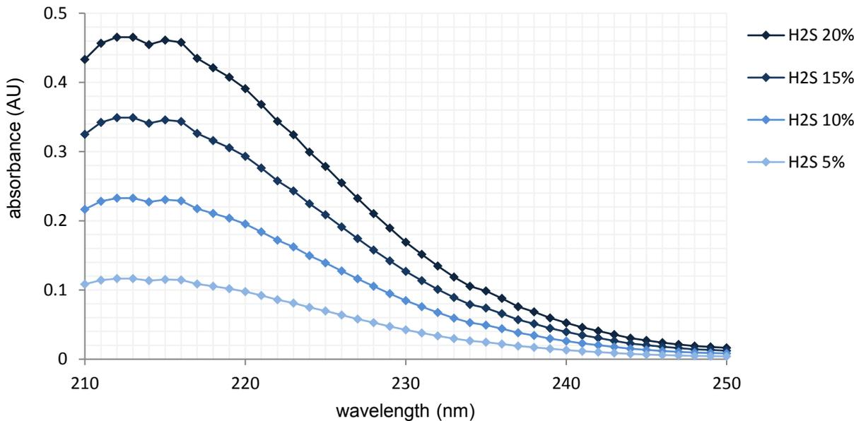
In the spectra above, each diamond represents a single photodiode and data point. The spectrophotometer measures absorbance at each integer wavelength within the 200-800 nm UV-Vis range and produces an H<sub>2</sub>S absorbance curve.
