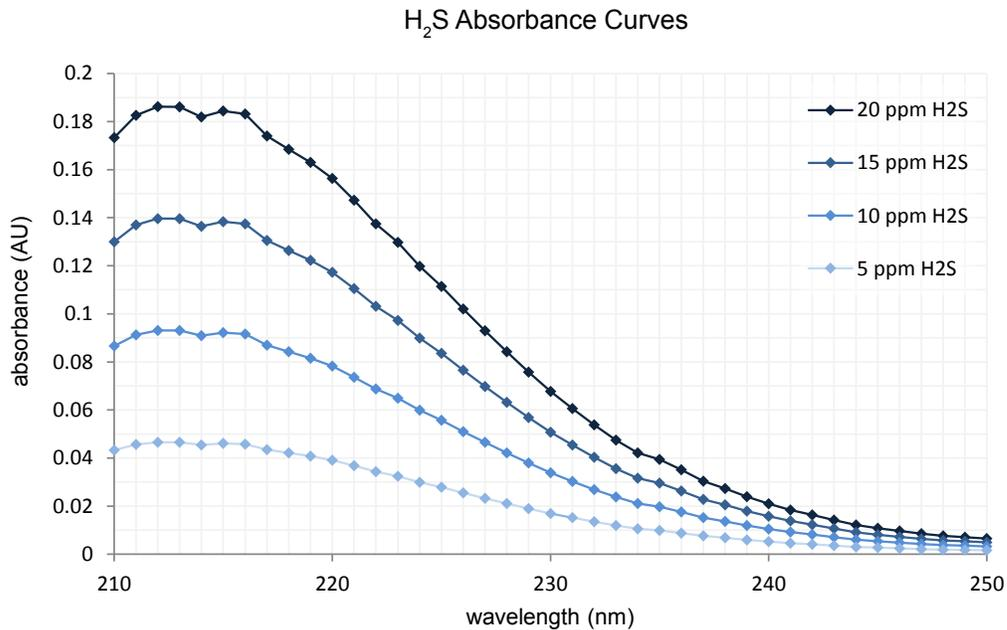
In the spectra above, each diamond represents a single photodiode and data point. The spectrophotometer measures absorbance at each integer wavelength within the 200-800 nm UV-Vis range and produces an H<sub>2</sub>S absorbance curve.
