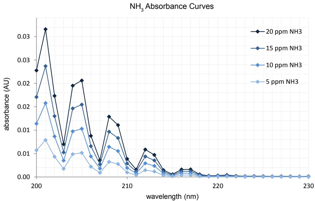
As with the H<sub>2</sub>S calibration explained above, the NH<sub>3</sub> analysis is calibrated on a full spectrum of standard NH<sub>3</sub> solution. In the double headspace configuration, each analyte has its own flow cell with path length specialized for the concentration range.
