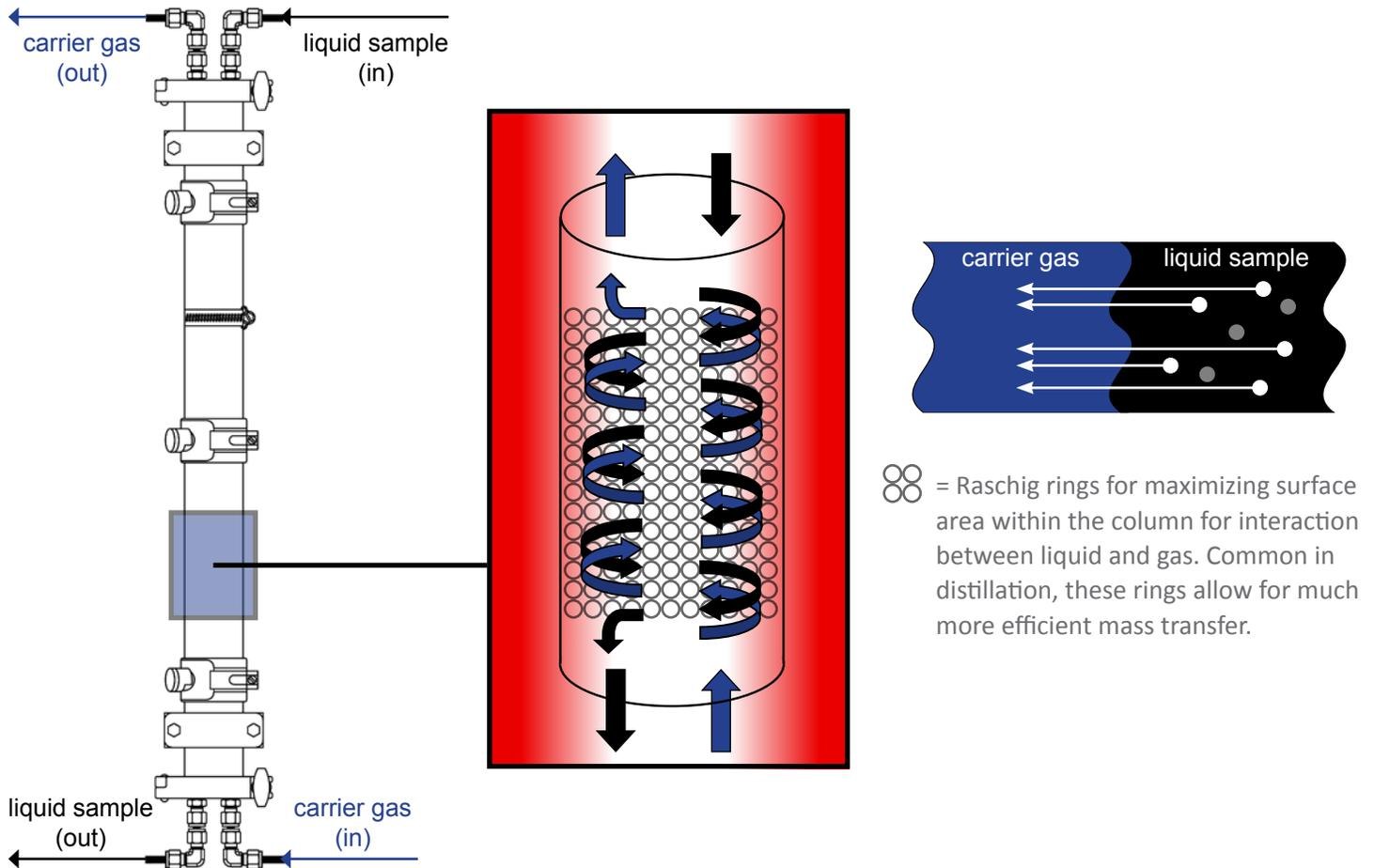
The held temperature determines the partial pressure mix of compounds in the headspace gas. This allows us to hold the temperature of the column at a point where we get an extremely useful vapor-phase sample that contains the analyte but very low levels of interfering compounds like aromatics and phenols (due to the difference in Henry's law constants between the analyte and the interfering compounds).
